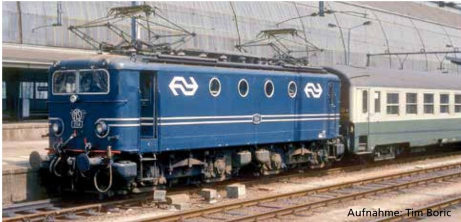
With the extensive electrification of railway lines in the Netherlands after the Second World War, electric locomotives had to be procured as quickly as possible by the Nederlandse Spoorwegen. The 60 new series 1100 electric locomotives ordered in 1948 are based on the original design of the French BB 8100.
