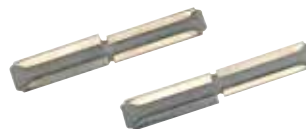
55293 Wide Rail Conversion Joiners, 6 pieces Rail joiners made of spring steel with two different end widths, make connection possible to the PIKO-Hobby track produced between 1992 and 2002, the Mehano* track, classic Roco* 0.1" (2.5 mm) track of brass and nickel, the Fleischmann Profi* – and model tracks and other tracks with 0.1" (2.5 mm) high profiles, 6 pieces.
